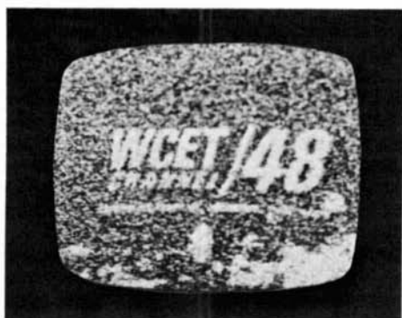
WCET, channel 48, Cincinnati, Ohio. A 255-mile tropo path.
